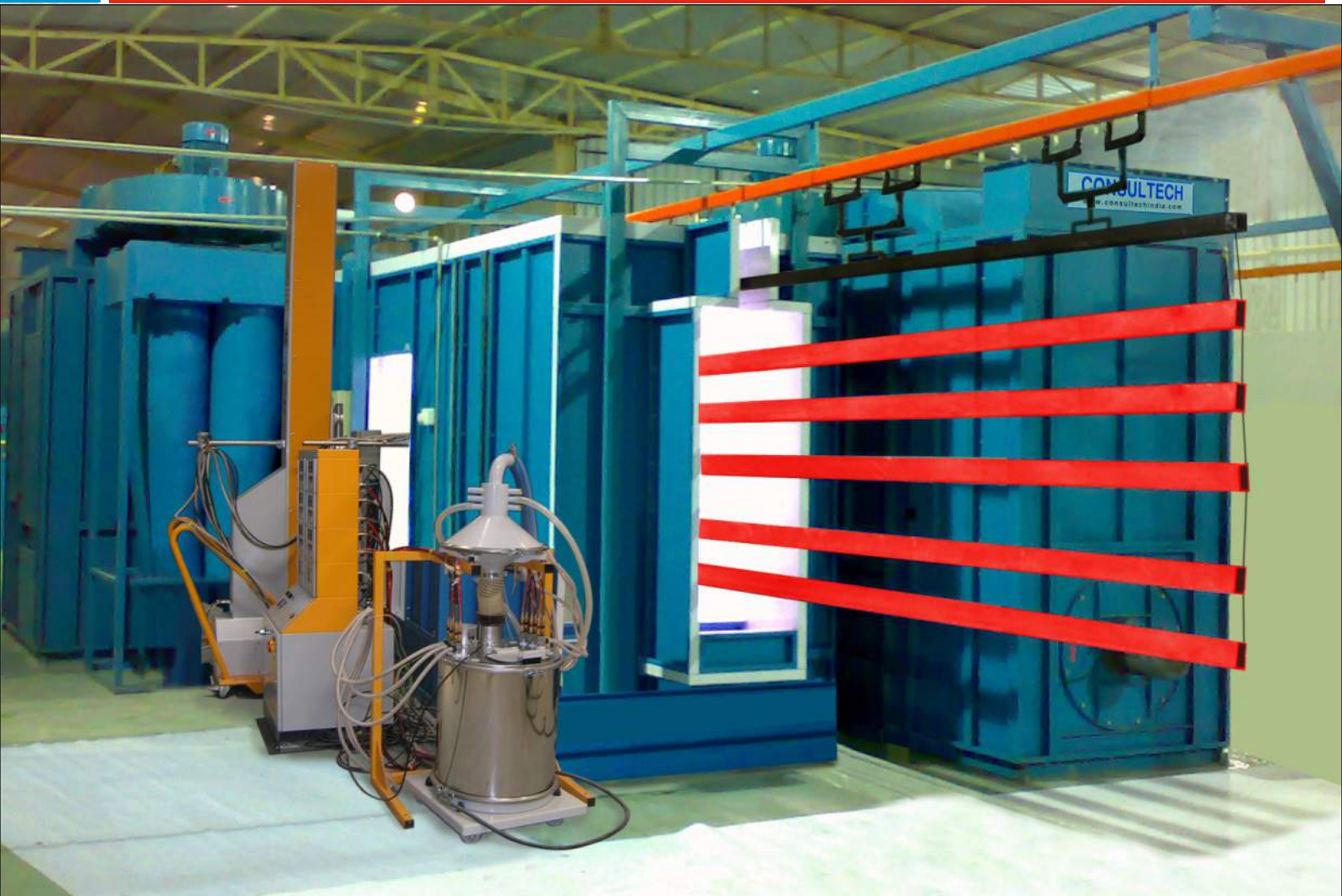
Conveyorised & automatic powder coating system
