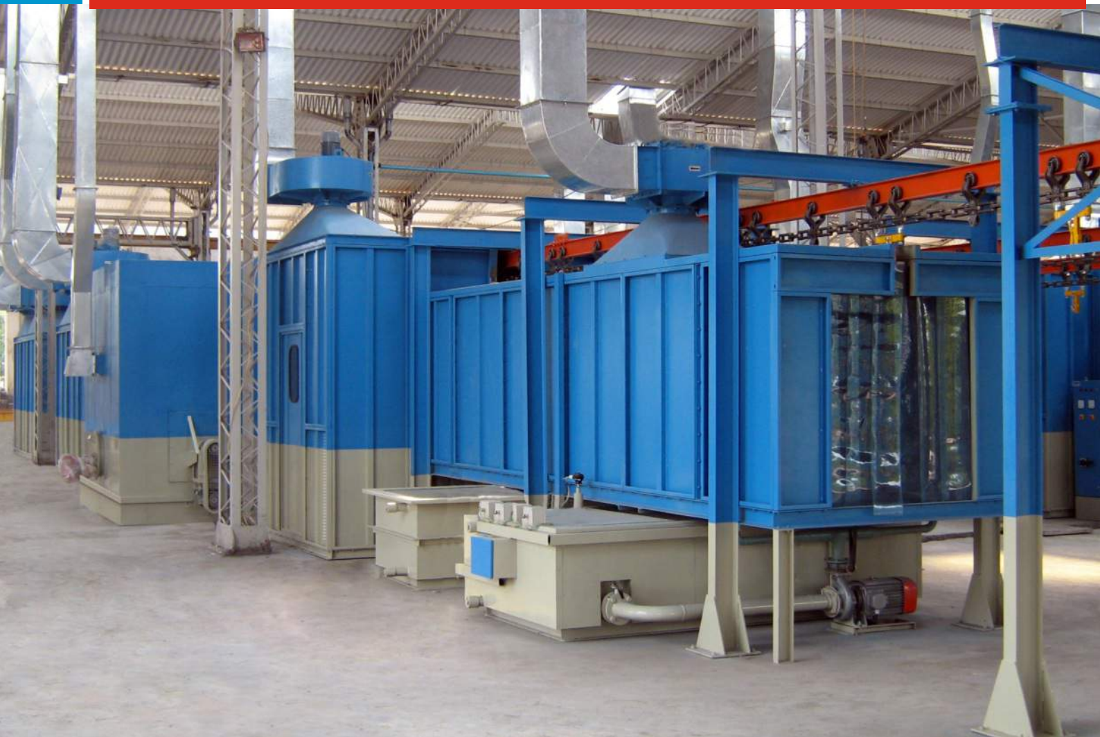
Conveyorised spray pre-treatment system
