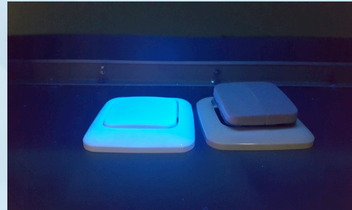
Coated vs. Uncoated (exposed to UV light)
